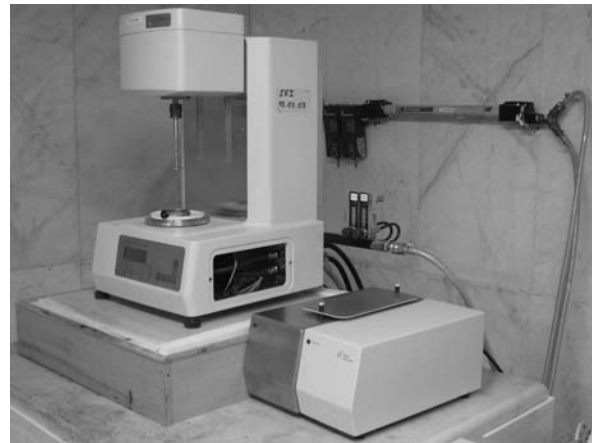
Fig. 2. MCR300 rheometer used for rheological measurement under magnetic field.
